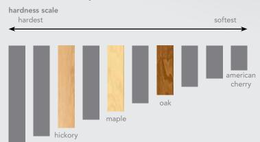
The density and hardness of wood products varies by species. The hardness of species scale can help determine the optimal wood selection.
