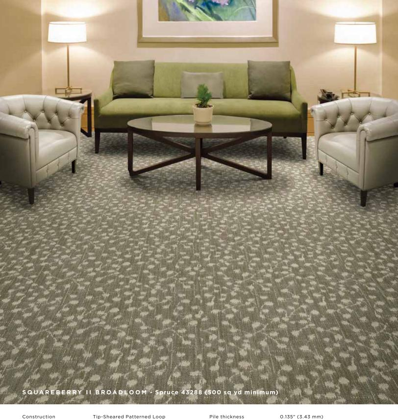
Tip-Sheared Patterned Loop Antron® Legacy™ Type 6,6 Nylon Solution / Yarn 5/64 (50.4 per 10 cm) 12.33 (48.54 per 10 cm) Pile thickness
